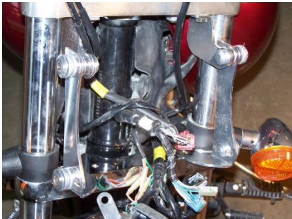
Brackets installed with headlight out.
