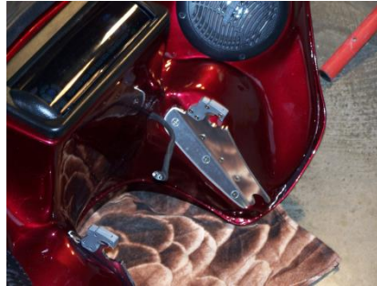
Looking down on the fairing with the Memphis Shade bracket installed.
