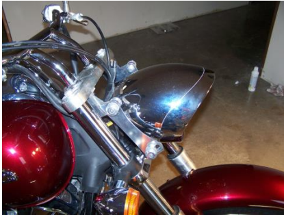
Side view of installed brackets and headlight reattached.
