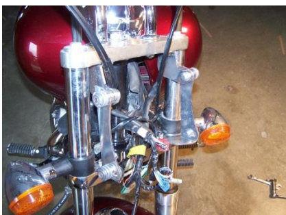
Side view of brackets installed and headlight off.
