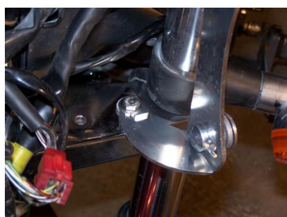
Looking down on the bottom of the triple tree where the 1/4" hole has been drilled and the bracket is installed.
